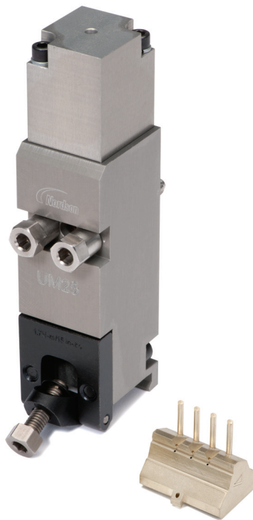
Nozzles detach easily without removing modules.
