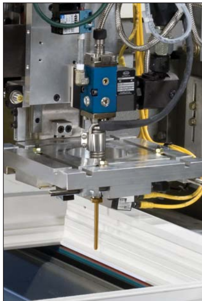
AG-900+ dispensing applicator in window backbedding application
