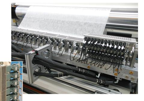
The patented Porous Coat system applies discrete, random and open patterns of hot melt adhesive to substrates in narrow- or wide-web applications. The unique surface application provides excellent bonding as well as reduces adhesive use and cost. Coated webs demonstrate soft hand and drape properties.
