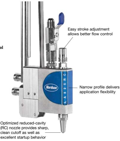
Nordson LA 825 RC electric guns are ideal for the small adhesive quantities, intermittent application, and high-line speeds found in folding carton production. The fast-cycling, non-contact guns maintain consistent adhesive deposition even during line speed changes.
