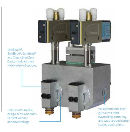
The PatternPro<sup>™</sup> gun features a rotating disk design, which allows you to rotate the modules on the gun body, easily creating new patterns and dramatically reducing downtime during product changeover.
