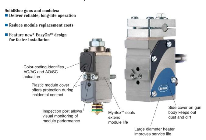
SolidBlue guns and modules are available in two designs. SolidBlue S guns feature air-open/spring-closed (AO/SC) and SolidBlue A guns feature air-open/air-closed (AO/AC) actuation. Both guns provide up to twice the service life of the industry standard Nordson H-200 series guns.
