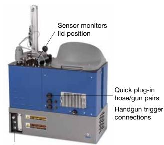
Flow-through output manifold with no dead spaces can accommodate up to three hoses
