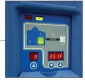
Melter controls automatically recognize and run optional hose/qun channels
